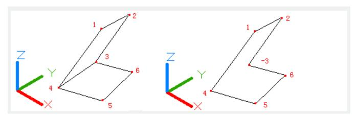
Polygon with arbitrary number of edges also could be created. The PFACE command could
