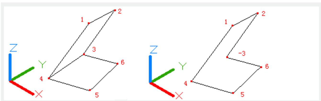
Polygon with arbitrary number of edges also could be created. The PFACE command could
