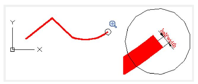
The halfwidth of start point will be default halfwidth of endpoint. The halfwidth of endpoint will become the sub-sequence default halfwidth for all segments until changed. The start point and the endpoint of wide lines lie in its center.
