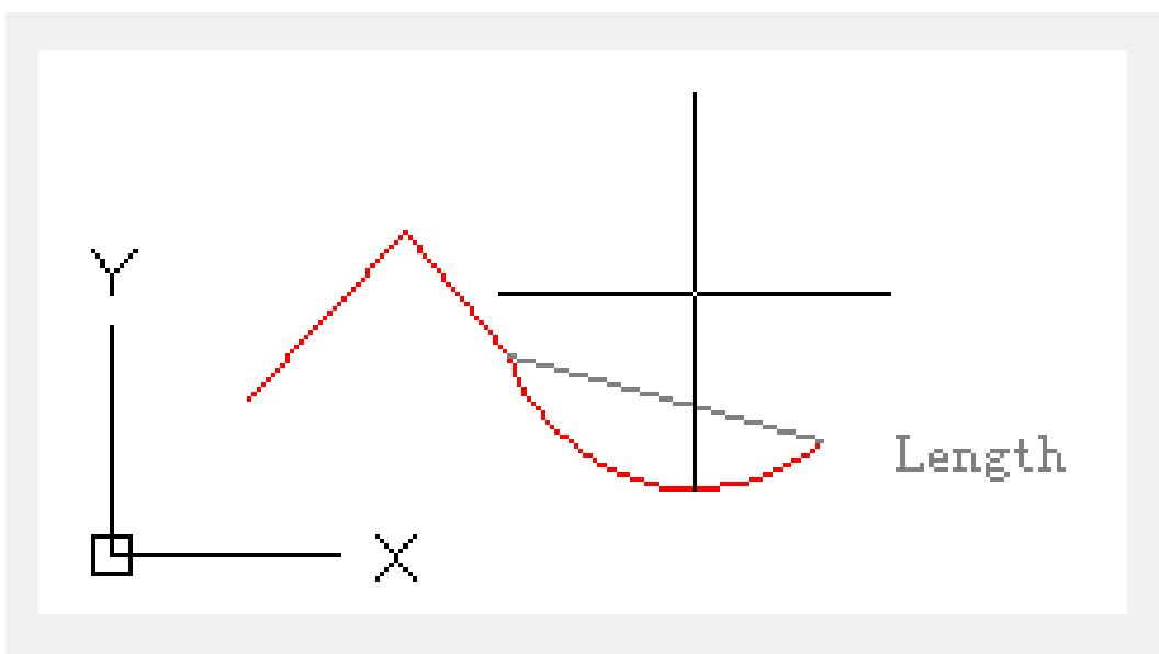
**Close** : Create an arc from the last point to the start point and form a close polyline. Users should select at least two points to create a polyline by this option.
