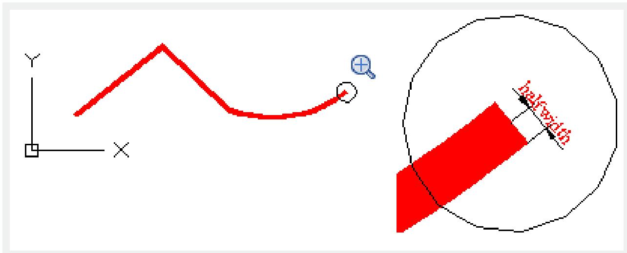
The halfwidth of start point will be default halfwidth of endpoint. The halfwidth of endpoint will become the sub-sequence default halfwidth for all segments until changed. The start point and the endpoint of wide lines lie in its center.
