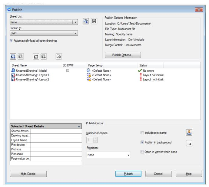
Inputting "\_publish" under the command prompt, the "Load sheet list" dialog box pops up. Users could select and open the existing drawing sets documentation (DSD), and then the "Publish" dialog box displays all saved and to be published drawing sets in DSD flies. Specifying the FILEDIA system variable to 0 and inputting "\_publish" under the command prompt, it will display options.
