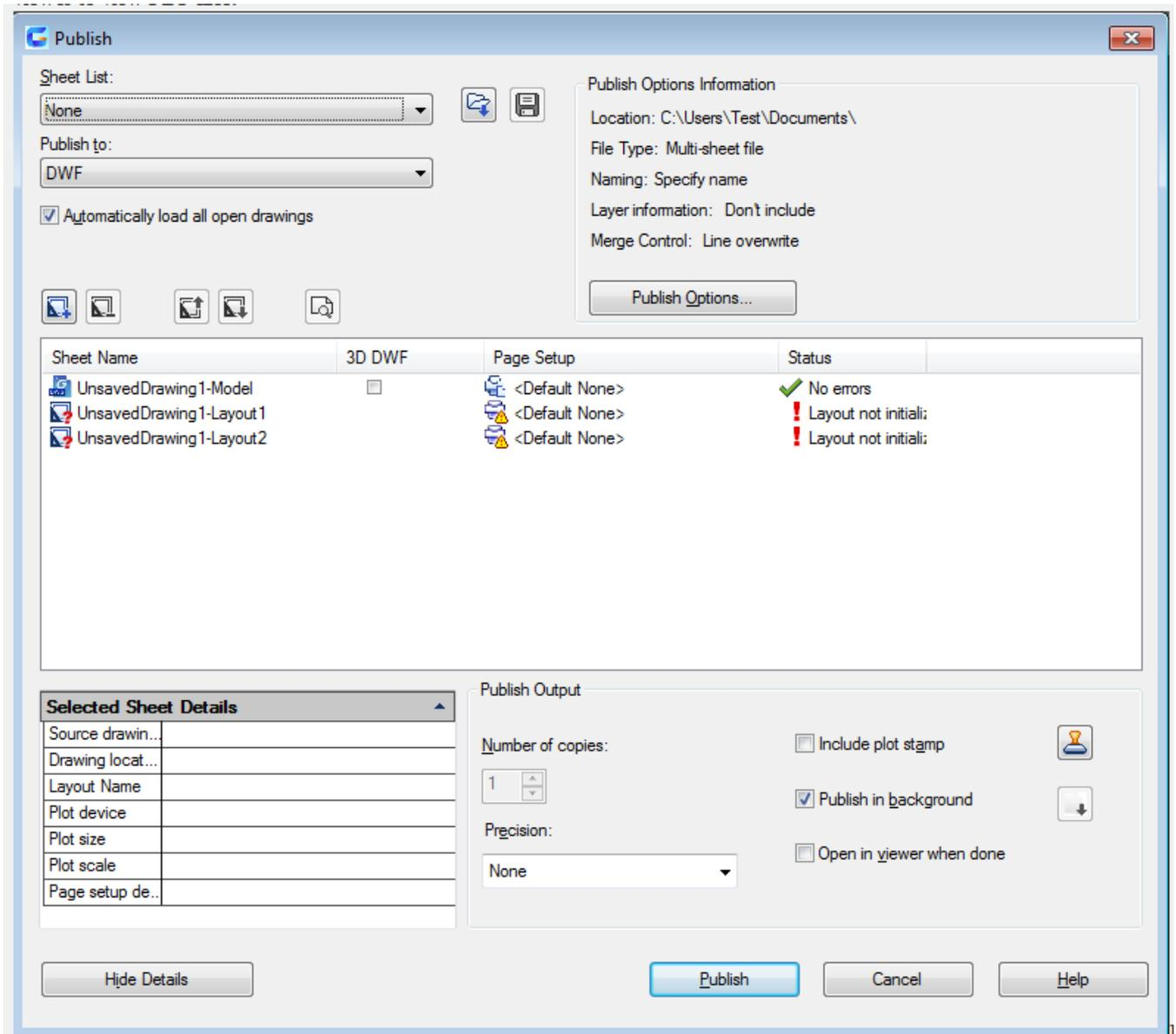
Inputting "\_publish" under the command prompt, the "Load sheet list" dialog box pops up. Users could select and open the existing drawing sets documentation (DSD), and then the "Publish" dialog box displays all saved and to be published drawing sets in DSD files. Specifying the FILEDIA system variable to 0 and inputting "\_publish" under the command prompt, it will display options.
