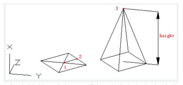
At first, the default base radius has not specified any value. During drawing, the default base radius is the previously used base radius. Users could select the "Top radius" option to create pyramid of flat section.
