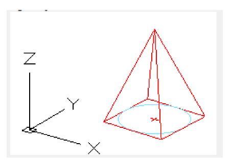
**2P :** Specify the height of pyramid to be the distance between two specified points. **Axis endpoint :** Specify the position of axis endpoint of pyramid. This endpoint is the vertex of pyramid and it could be any position in 3D space. The axis endpoint defines the length and direction of pyramid
