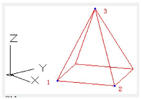
**Sides**: Specify the number of sides. Users could specify a number from 3 to 32. At first, the number of sides is specified to 4, during drawing, the default number of side is the previously inputted value.
