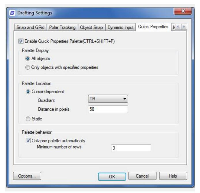
**Enable the Quick Properties Palette:** Displays the Quick Properties palette when you select objects. **Palette Display:** Sets the display settings of the Quick Properties palette.
