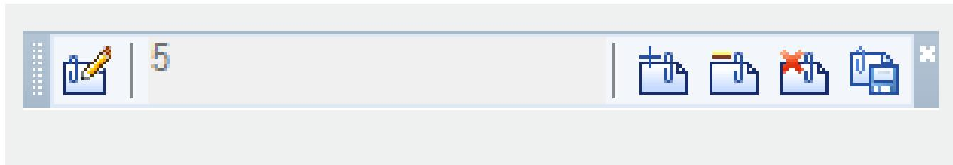
This command could extract specified objects from an external reference or a block and make it available to edit. The extracted objects are called working set, users could modify and save the working set to refresh external reference or block definition. Inputting "\_refedit" under command prompt, it will display options.
