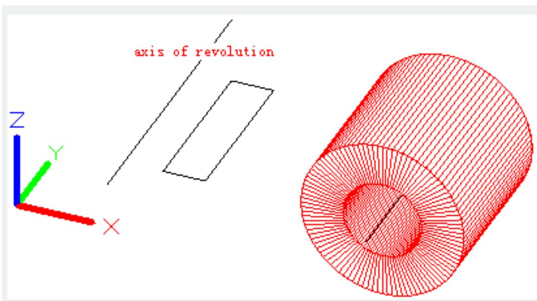
The object will be swept around selected axis to create meshes. Users could create closed meshed by selecting circle or closed polyline as sweeping trace. The axis of revolution is determined by the vector that defined by the first vertex directs to the end vertex, all middle vertexes will be ignored.
