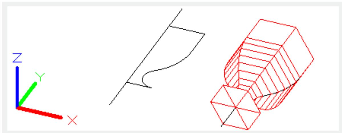
Users could create meshes by selecting straight line, arc, circle, 2D polyline or 3D polyline. They could also revolve them by specified axis along sweep trace. The MESHTYPE system variable could specify the mesh type. By default, it is specified to 0 for creating polyface meshes or polygon meshes.
