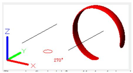
The rotation direction is influenced by the selecting point on axis of revolution. On the following are two examples:
