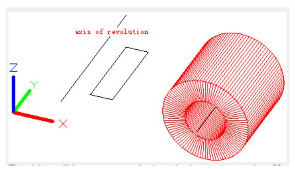
The object will be swept around selected axis to create meshes. Users could create closed meshed by selecting circle or closed polyline as sweeping trace. The axis of revolution is determined by the vector that defined by the first vertex directs to the end vertex, all middle vertexes will be ignored.
