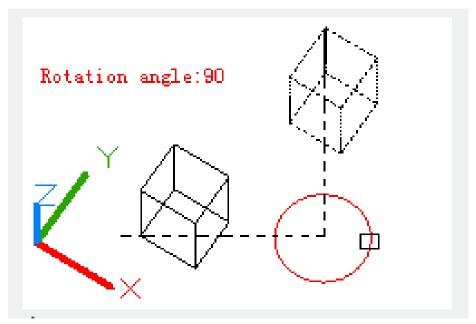
**Arc**: Align the rotation axis to the 3D axis of arc (the rotation axis goes across the arc center and is perpendicular to the arc plane).
