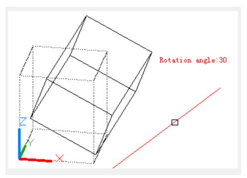
**Circle**: Align the rotation axis to the 3D axis of circle (the rotation axis goes across the circle center and is perpendicular to the circle plane).
