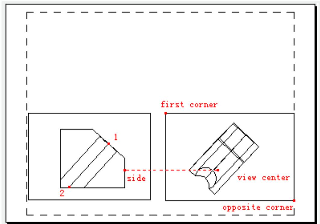
Create a section plane by two points in original viewport. Specify the side of view by selecting one point. Users could scale viewport by inputting view scale, the default value is 1, the scale factor is equal to zoom  $1.0 \times p$ . Users could define the view center under the prompt of "specify view center". Press ENTER to accept the default scale, the vertical line appears to guide locating the view center; otherwise, users could place the section view at any position.
