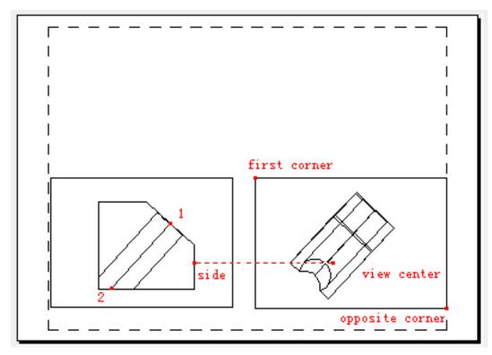
Create a section plane by two points in original viewport. Specify the side of view by selecting one point. Users could scale viewport by inputting view scale, the default value is 1, the scale factor is equal to zoom 1.0×p. Users could define the view center under the prompt of "specify view center". Press ENTER to accept the default scale, the vertical line appears to guide locating the view center; otherwise, users could place the section view at any position.
