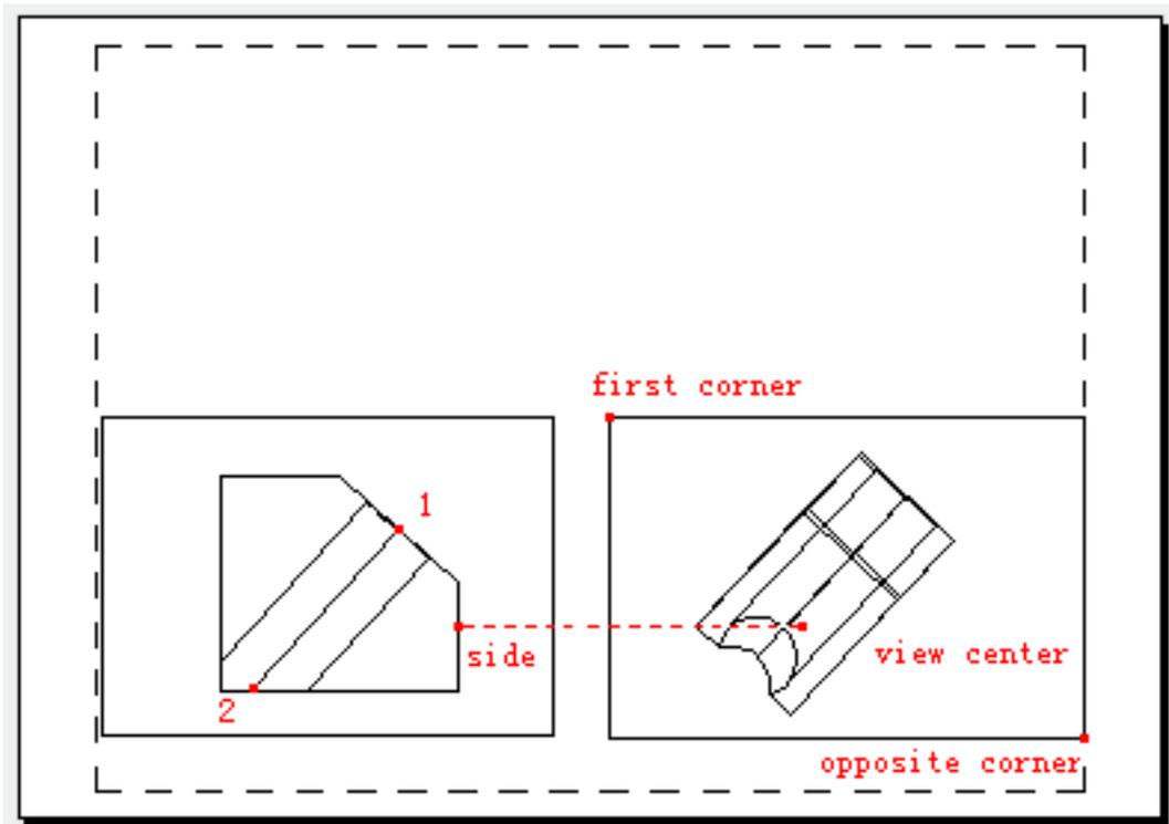
Create a section plane by two points in original viewport. Specify the side of view by selecting one point. Users could scale viewport by inputting view scale, the default value is 1, the scale factor is equal to zoom 1.0x. Users could define the view center under the prompt of "specify view center". Press ENTER to accept the default scale, the vertical line appears to guide locating the view center; otherwise, users could place the section view at any position.
