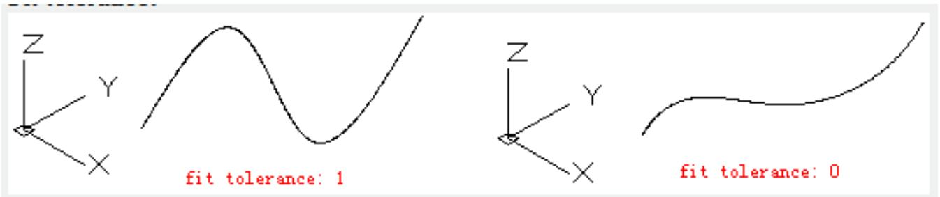
Specify the offset of fit points of a spline. If the fit tolerance is 0, the created spline goes through all fit points. The fit tolerance is applied on all fit points (except the start point and the end point).
