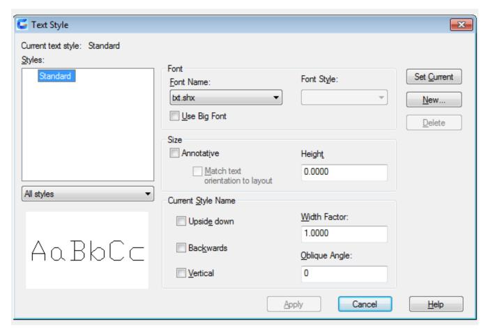
Inputting "-style" under the command prompt, it will display options. Users could set the current text style to determine the new one. The text style contains the font, size, oblique angle, direction and other features.
