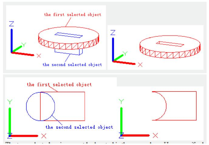
The two selected regions must be located in the same plane. However, if selected several regions on different plane sets, it will execute several times of SUBTRACT commands. If there is no overlapped region, the SUBTRACT will be refused. The SUBTRACT command could not be applied on mesh objects. If selected mesh objects, it will prompt to convert them to 3D solids or surfaces.
