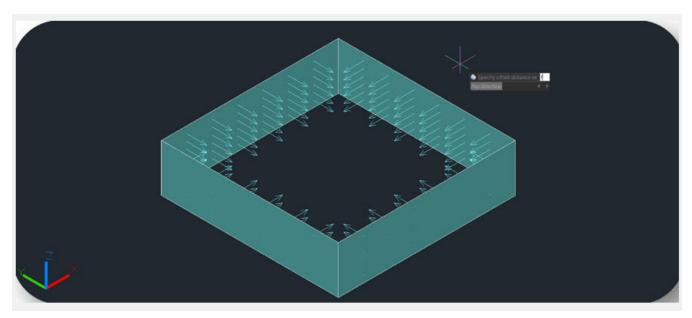
If you type "Both sides", you can Offset the surface in both directions (the arrows will show on both sides of the surfaces)
