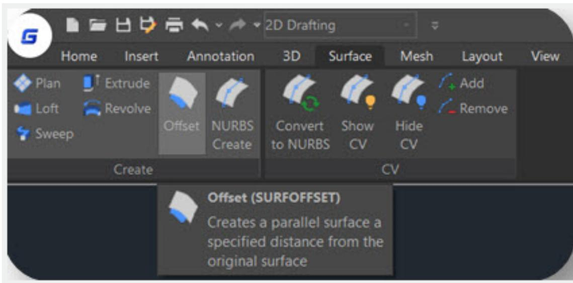
After selecting the surface and pressing enter, you will get 4 options (Flip direction, Both sides, Solid, Expression) in the command line and dynamic input box.
