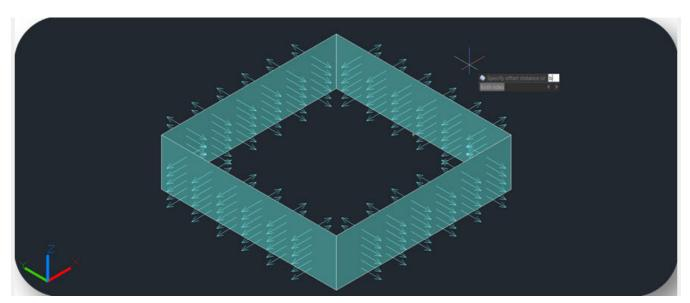
If you type "Solid", you can Generate the surface to a solid after the offset
