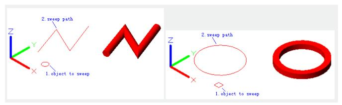
The following objects could be used to sweep: 2D or 3D spline, 2D polyline, 2D solid, edge sub object of 3D solid, arc, circle, ellipse, elliptical arc, line, region, solid, edge sub object of solid, surface and mesh, wide line. The following objects could be used as sweeping path: 2D or 3D spline, 2D or 3D polyline, edge sub object of 3D solid, helix, arc, circle, ellipse, elliptical arc, line.
