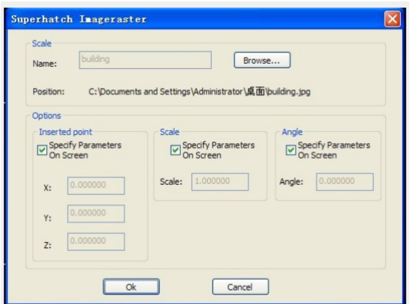
3. Pick the OK button in the Superhatch Imageraster dialog box, specify insertion point, scale factor and angle of rotation.
