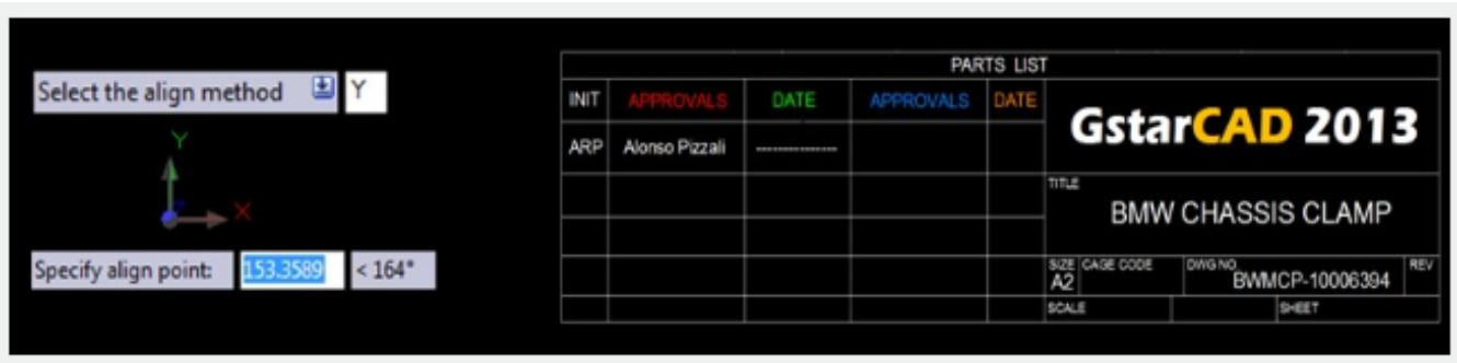
In another example, we choose the X axis alignment method and then specify a point to align the texts in the correct location (end point of Leader). The result is as follows:
