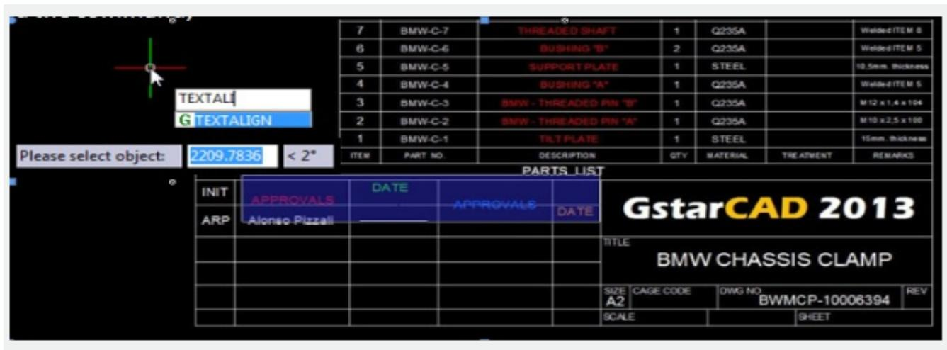
After selecting the text(s), a message will display > Select the align method: X axis (X) / Y axis (Y) / Two points (P):
