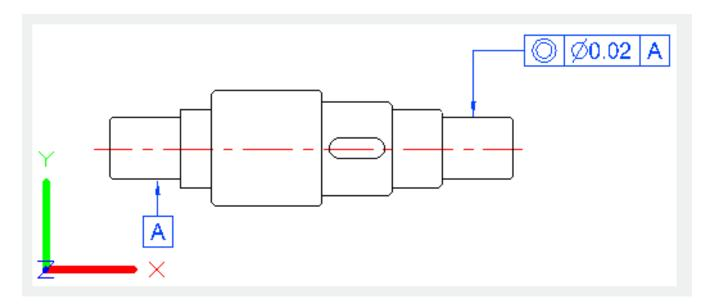
The TOLERANCE dialog box is used to specify the symbols and values for a feature control frame.
