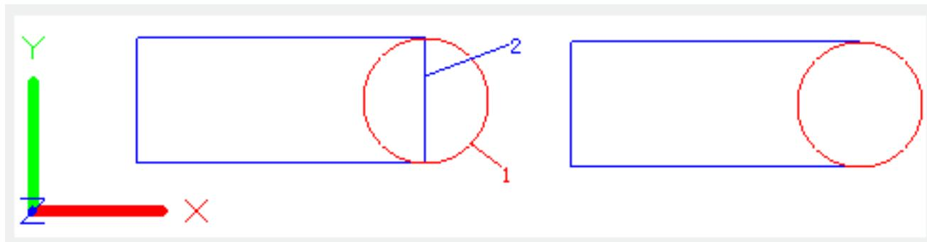
Select boundary of object to be trimmed or press ENTER to select all displayed objects as potential boundaries. The TRIM command will project the boundary and objects to be trimmed into XY plane of current UCS.
