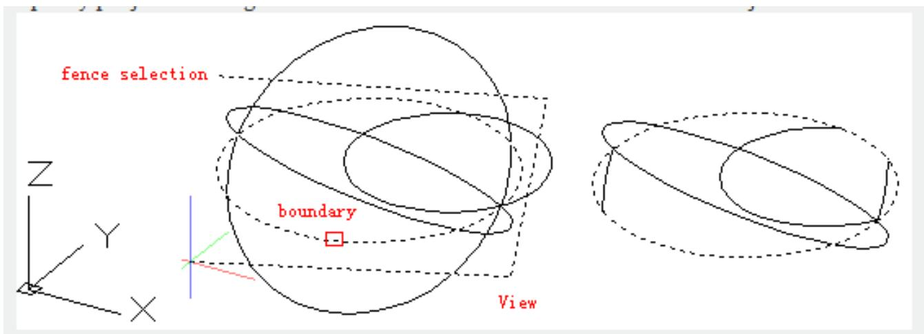
**Edge** : Determine to trim the object at the intersection in 3D space or on its extended edge.
