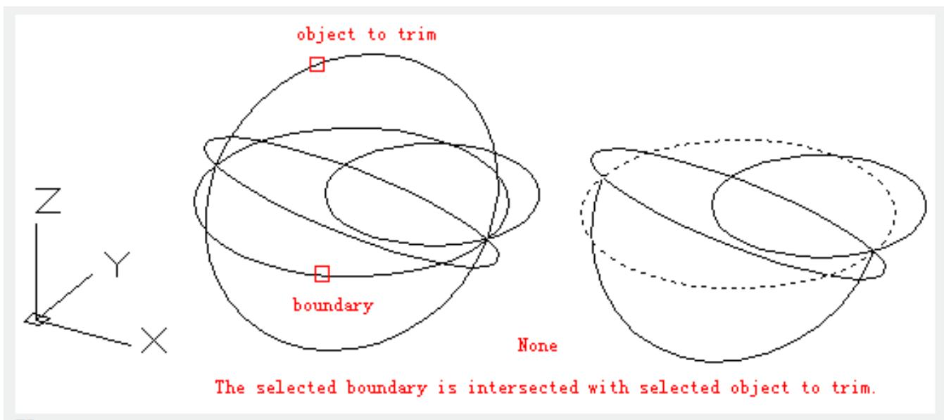
**UCS** : Specify projection on the XY plane of current UCS. It will trim objects that intersected with selected boundary on the XY plane in current UCS. Objects without intersection with selected boundary will not be trimmed in 3D space.
