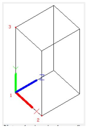
**Note**: when inputting the coordinate, if there is no specified Z coordinate, it will use the current Z value. **Face**:
