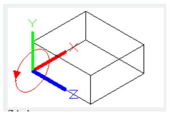
**Z** axis: Align the UCS to the specified Z axis.
