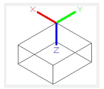
**Object:** Move the UCS to be tangent at specified point of selected object and align the origin to its endpoint. The positive direction of Z axis is deviating from selected object.
