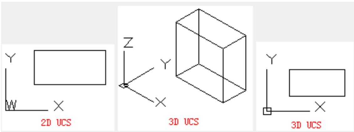
**3D**: if the current UCS is the same as WCS, looking down the UCS (the positive direction of Z axis), the origin in XY plane displays as a box; looking up the UCS, the box disappears.
