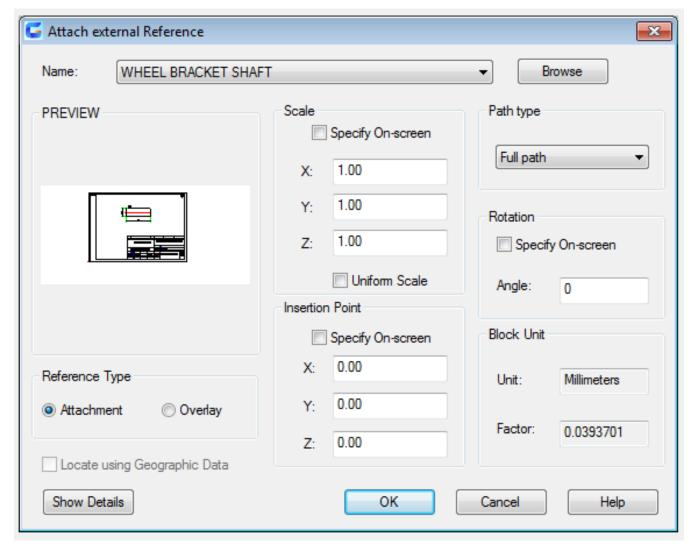
When attaching the metafiles in current drawing as external reference, it could also be linked to current drawing. Open or reload the reference drawing, the current drawing will display all modifies. Inputting "XATTACH" in command line, the "select reference file" dialog box pops up, and then select the specified DWG file, the "Attach External Reference" dialog box displays.
