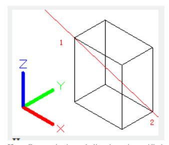
**Hor**: Create a horizontal xline through specified point. This xline is parallel to X axis.
