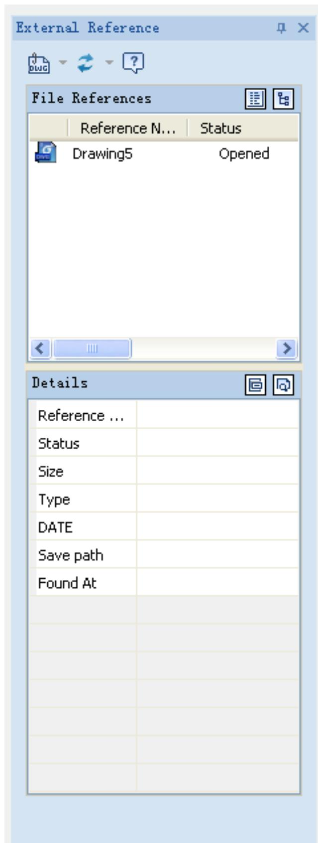
The Xref Manager dialog box is used to edit and control external reference in current drawing.
