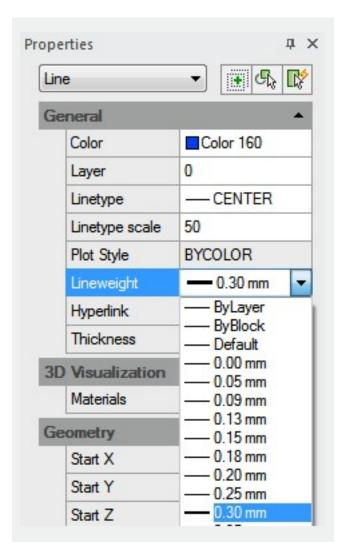
Usually the objects are created with the lineweight assigned to the current layer. If the current lineweight is set to BYBLOCK, objects are created with the default lineweight setting until the objects are grouped into a block. If you do not want to use the lineweight currently assigned to the layer, you can select any other lineweight for object.
