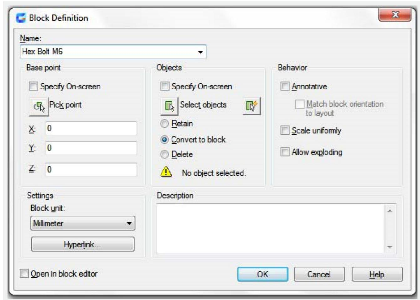
The base point is used as a reference for positioning the block when you insert it.
