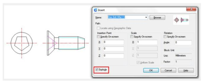
When you explode a block with nested block, only the top-level block will be exploded, the nested block not be exploded.
