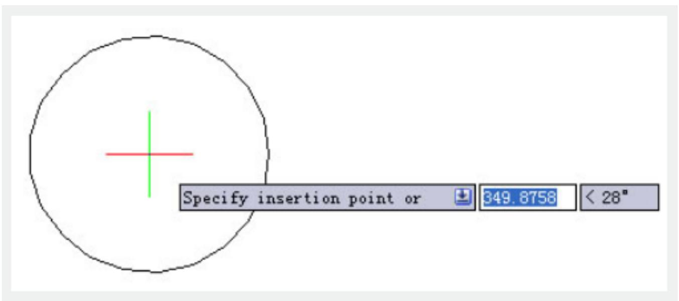
You can realize, base point becomes the insert point of the block after adding the base point parameter. Please note, if you set an insert point via the block define dialog box, and add a base point parameter as well, the base point is the default insert point.
