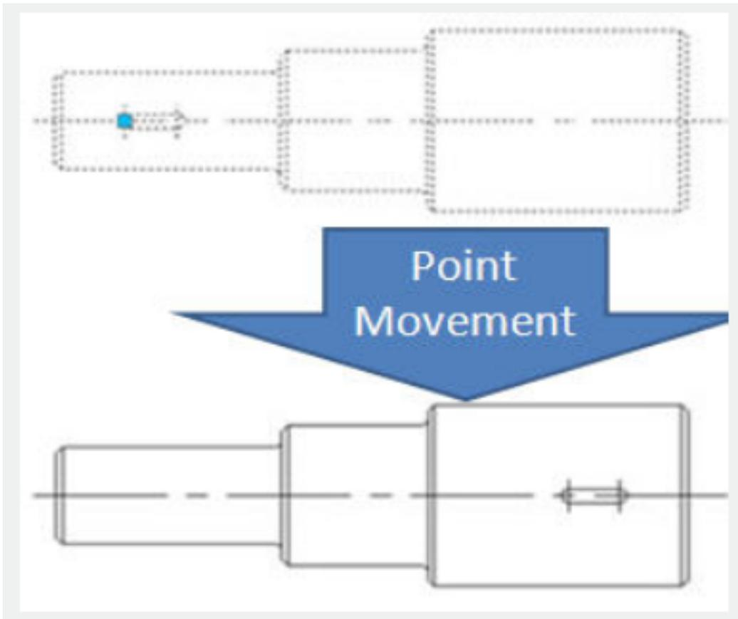
Please pay attention, if it is not run with orthotropic constraint, the keyway can move towards every direction because the direction of the point parameter is random, the characteristic of the parameter decides the characteristic of action.
