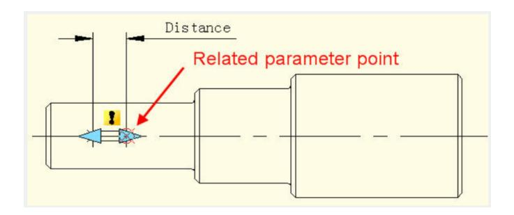
The parameter point we mentioned corresponds to the operate point of Move. After exiting Block Editor you can drag this point to make dynamic block change correspondingly.
