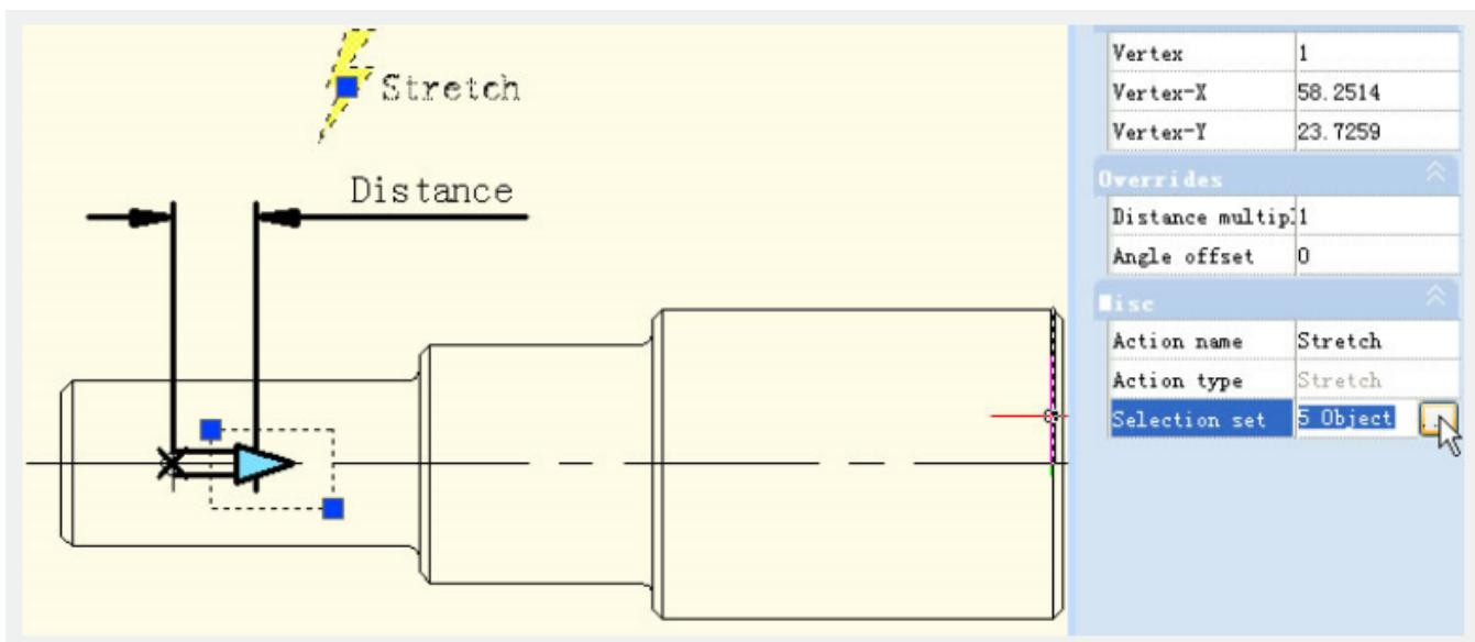
The black object is the operational object of the action, the broken line frame is the stretch frame, objects intersect with stretch frame will be stretched, objects which will be selected by the stretch frame will move.
