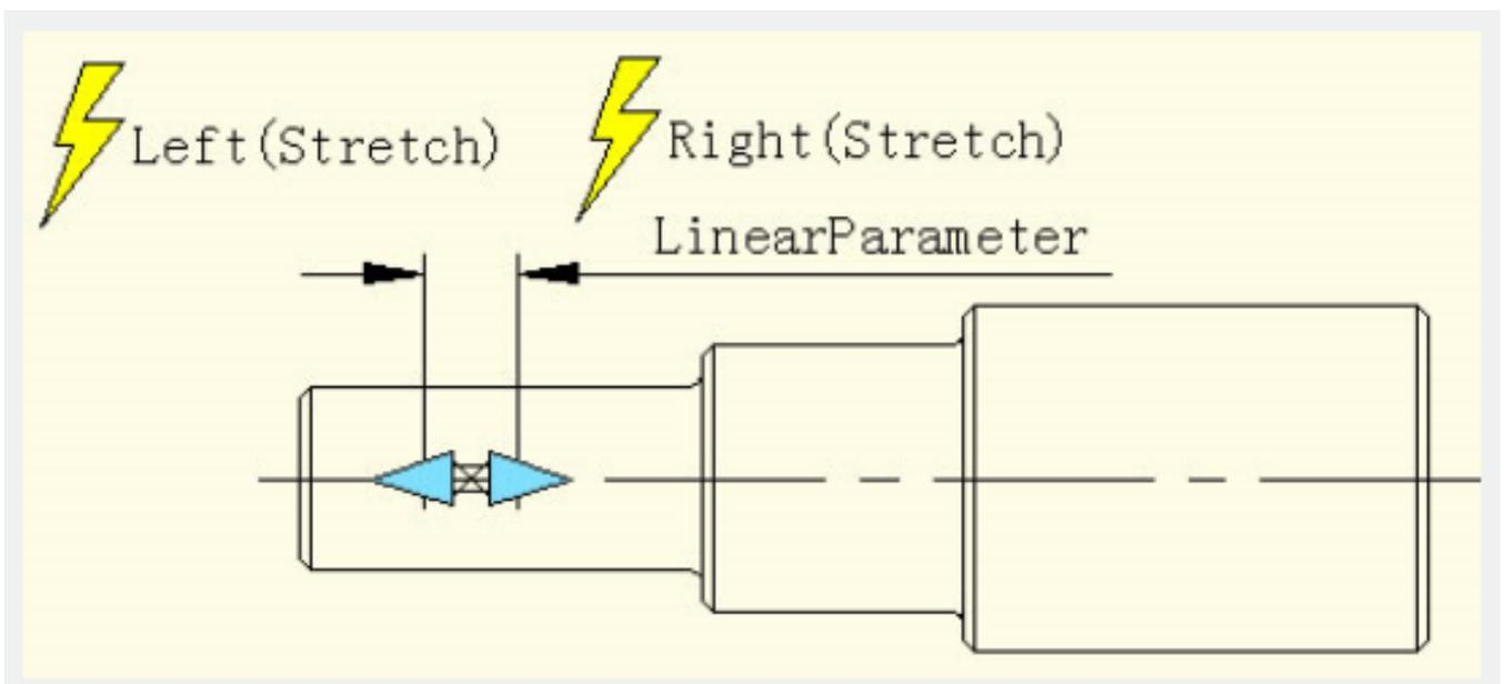
For the convenience of watching the effect, we drew a vertical center line in the middle of the keyway, and then stretched the grip to the left side of the keyway or the right side, as shown in the picture below. As the grips are moving, the two-way symmetrical stretch is realized.
