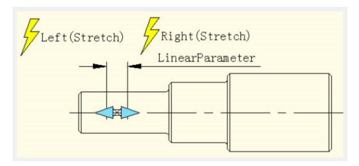
For the convenience of watching the effect, we drew a vertical center line in the middle of the keyway, and then stretched the grip to the left side of the keyway or the right side, as shown in the picture below. As the grips are moving, the two-way symmetrical stretch is realized.
