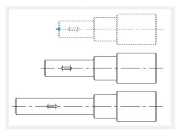
Although Stretch and Move have a common parameter, when the Distance Multiplier of Move is modified to 0.5, the displacement of Move can only stretch 0.5 times of the displacement.
