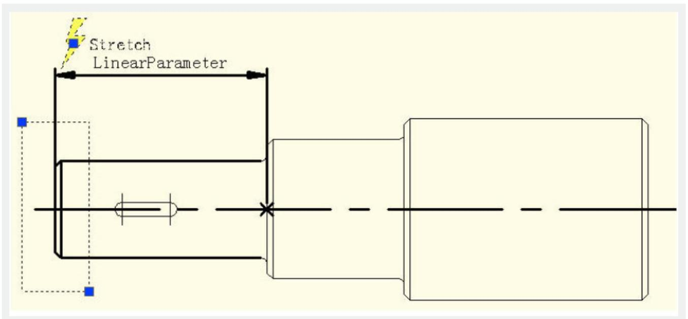
Because the follow-up operation will not stretch the step shaft by grips of this linear parameter, the grip's number of the linear parameter can be modified to "0".
