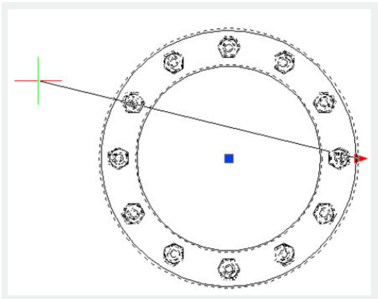
The reason for this is that the Endpoint of the Linear Parameter can not cross its base point, so we change the Linear Parameter to be a Polar Parameter, we do not change any other operations, as shown in the following picture.
