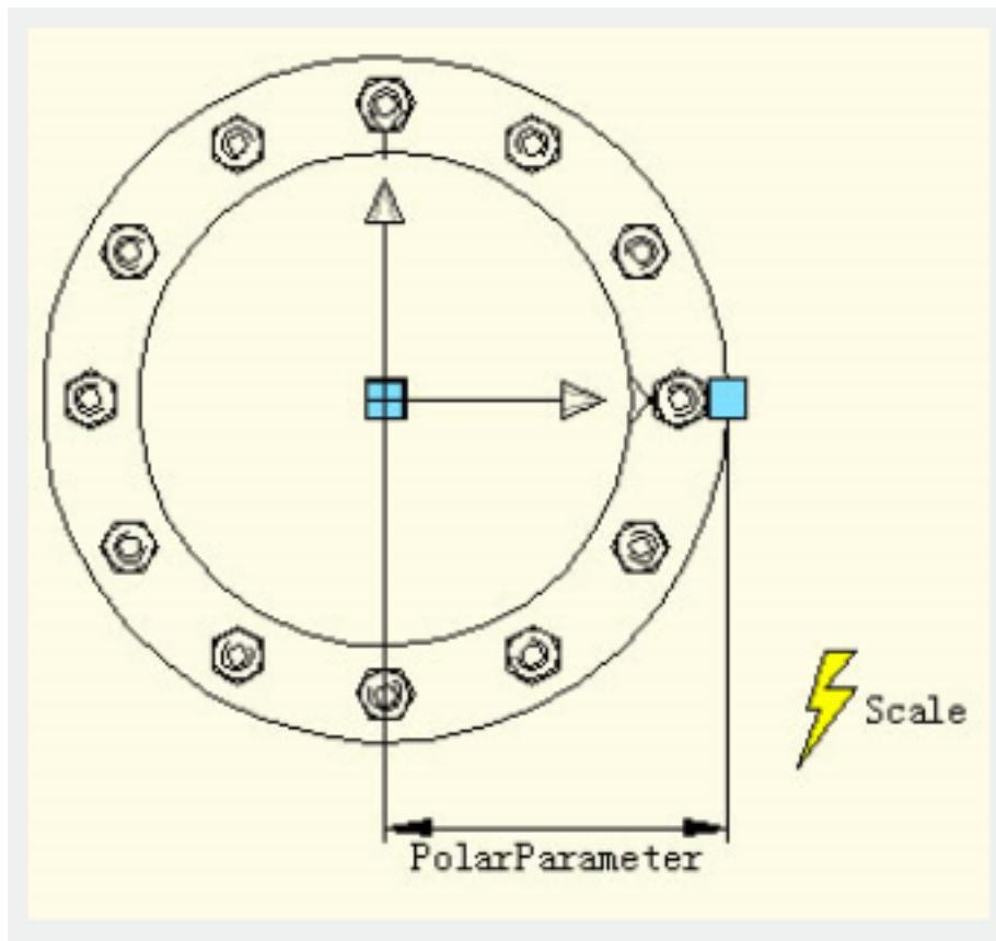
Exit from Block Editor, Drag the grips of the Access hole Block again, you can see, that after the change from Linear Parameter to Polar Parameter, we can drag the grip to scale the dynamic block in any direction.
