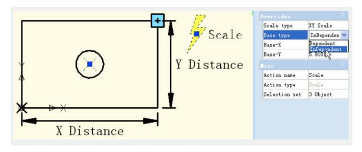
Specify new base: Single click the right input box of "Base-X" and "Base-Y", you can manually input the
