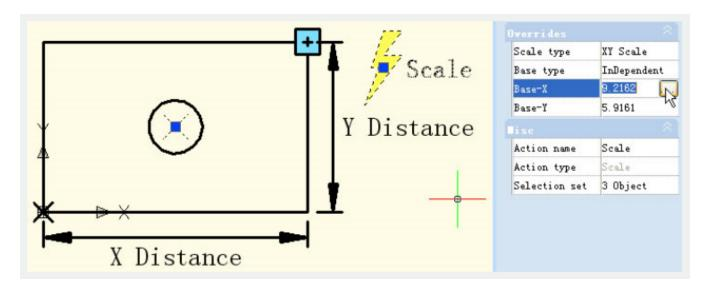
Specify the base point by crosshair and the circle center as base point. After exiting Block Editor, scale the dynamic block, the result will be as shown below:
