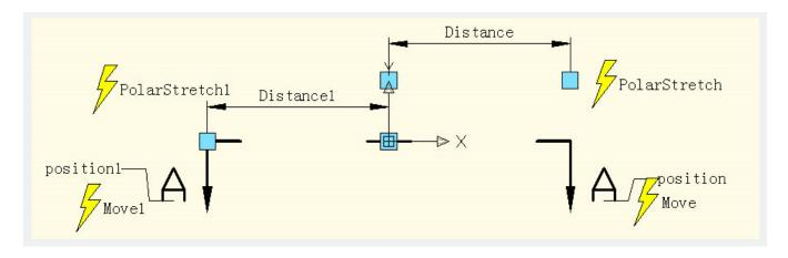
Exit block editor, move the right grip and you can see that rotate center moves up along with the parameter, as shown in the following picture.
