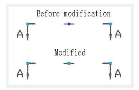
Clicking central grip can move the grip to any direction. Meanwhile, the dark blue insert point of block will appear again, as shown in the following picture. Obviously, the insert point is only covered by the base point of the polar parameter. The base point of the polar parameter can move arbitrarily, but for the block it seems that no change is happening. But is it true?
