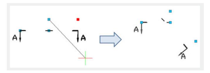
From the examples above it is difficult to understand that the polar parameter cannot move arbitrarily like the point parameter and linear parameter, the reason is that the base point of the polar parameter specifies the rotate center of the object, once the parameter is moved, the rotate center will move accordingly. That the rotate parameter cannot move arbitrarily has the same reason.
