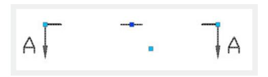
In order to confirm if the block changes or not, we move the grips on both terminals and we can find that the section symbol does not center on the dark blue base point when changing but it takes the base point of the polar parameter as a rotate center, as shown in the following picture.
