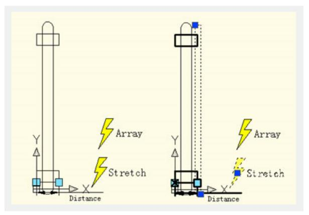
The Polar Parameter determines the way of Array directly, the Polar Array will regard the direction of the Polar Parameter as Array direction, achieving Array functions in any direction.
