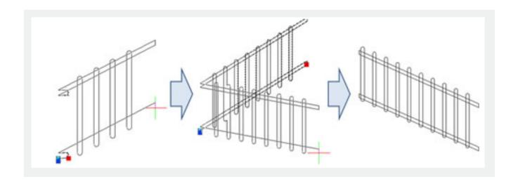
You can see, not only can we stretch the fence, but we can also rotate the direction casually, this is the effect combining Polar Stretch with Polar Array.
