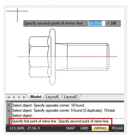
By default, Mirrored text, attributes and attribute definitions (<u>ATTDEF</u>) will have the same alignment and justification as before mirrored, they are not flipped. If you set the <u>MIRRTEXT</u> system variable to 1, text will be flipped
