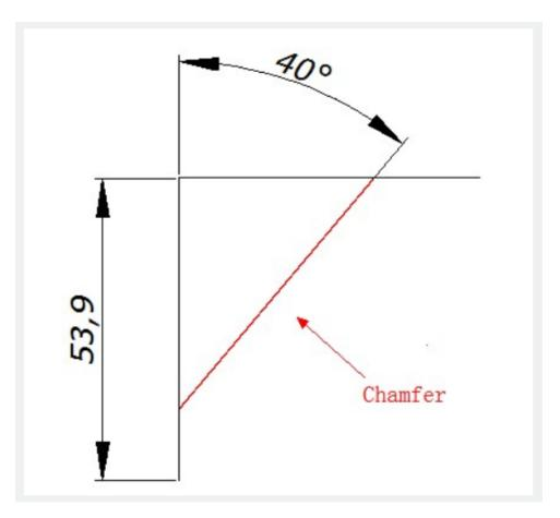
You can specify chamfer length on the first line and angle of chamfer instead of distances..
