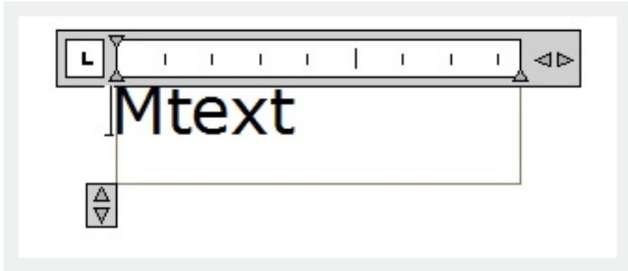
You can create mtext in the In-Place Text Editor or an alternative text editor, you can also insert text from a file. The In-Place Text Editor displays the bounding box with a ruler at the top and the Text Formatting toolbar.
