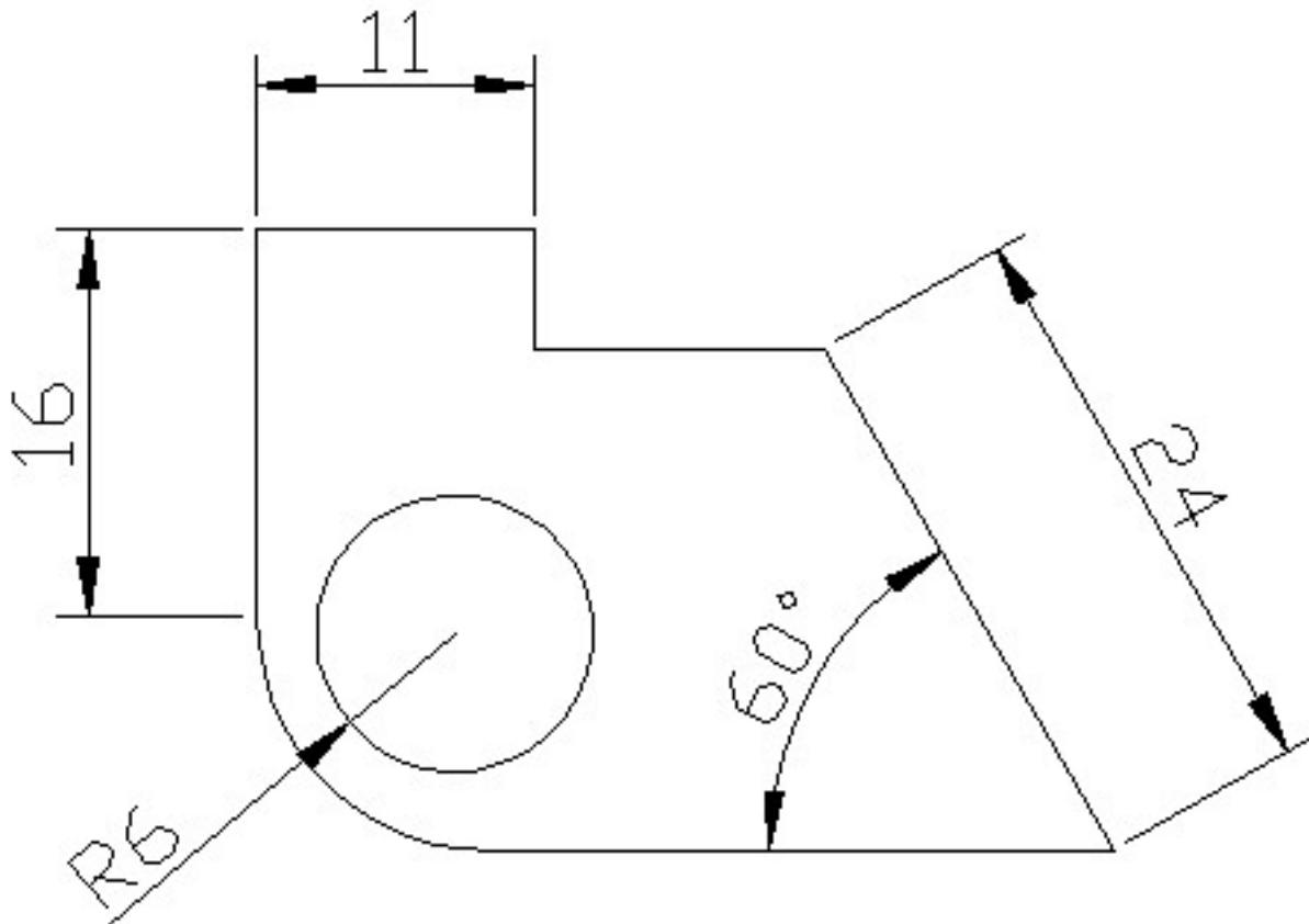
Dimensions have several elements: dimension text, dimension lines, arrowheads, and extension lines.
