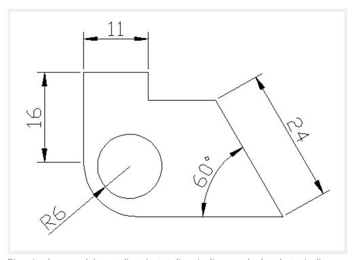
Dimensions have several elements: dimension text, dimension lines, arrowheads, and extension lines.
