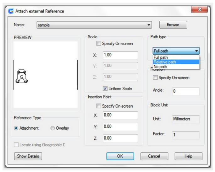
When you attach an external reference, its elements like layers (XREF), linetypes (LINETYPE), text styles and other elements are not added to the current drawing, but also linked from the referenced file.
