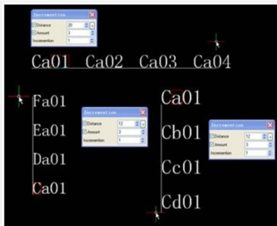
Free Incremental: It is used when the Incremental Copy location is relatively free, for example: number of spare parts in the assembly drawing.
