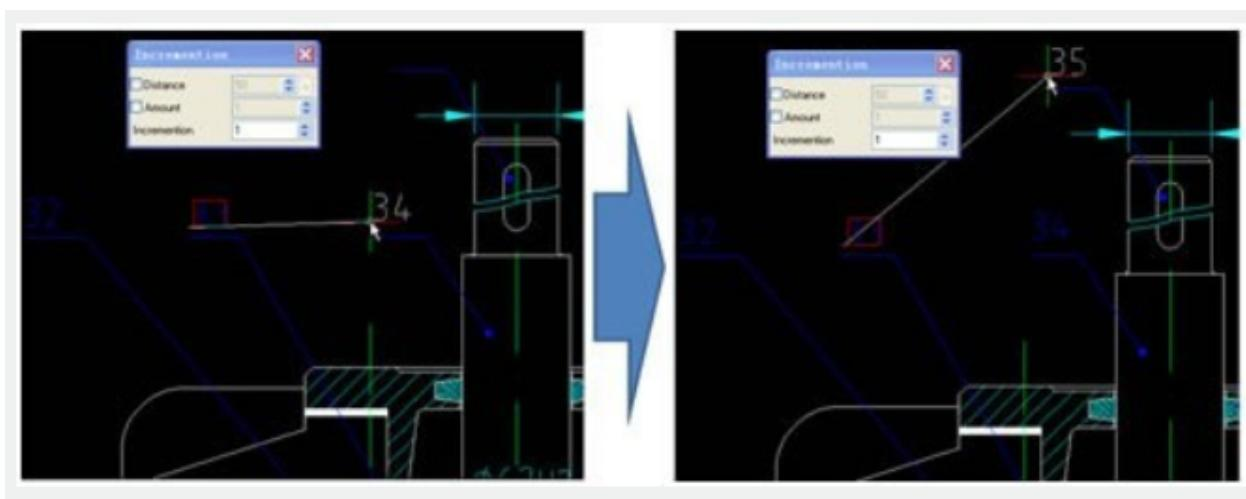
Distance only: It is used if the distance of incremental text is fixed, for example: number column in the form.
