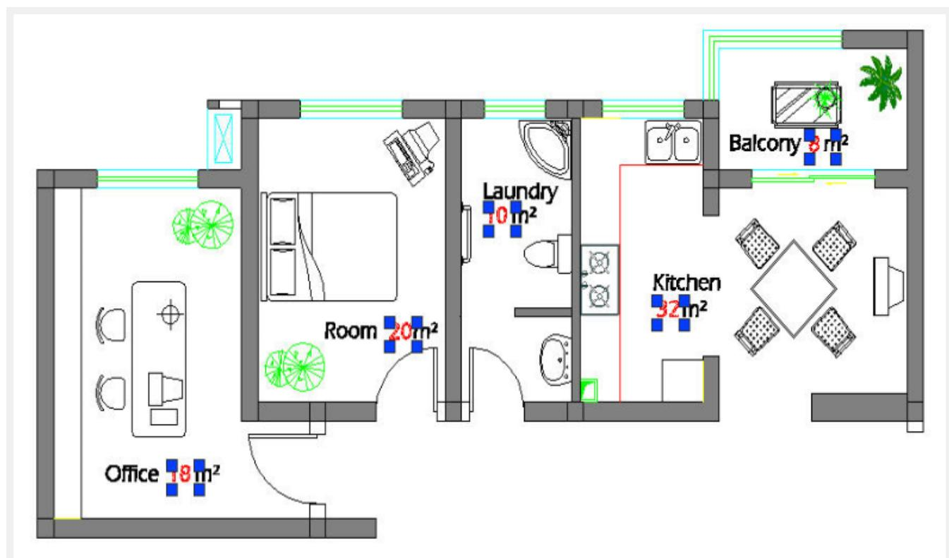
In the Statistics dialog box, you can see the cumulative sum from the selected text numerical values. You can also re-select, replace, copy text numerical value again plus fill-in (show) the cumulative sum in any point of your current drawing.
