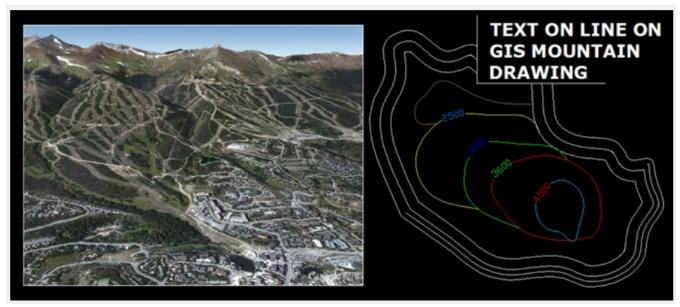
In the previous version, text online just allowed to overwrite text over one object. Now you can create text online quickly for multiple curves without performing the same command each time.
