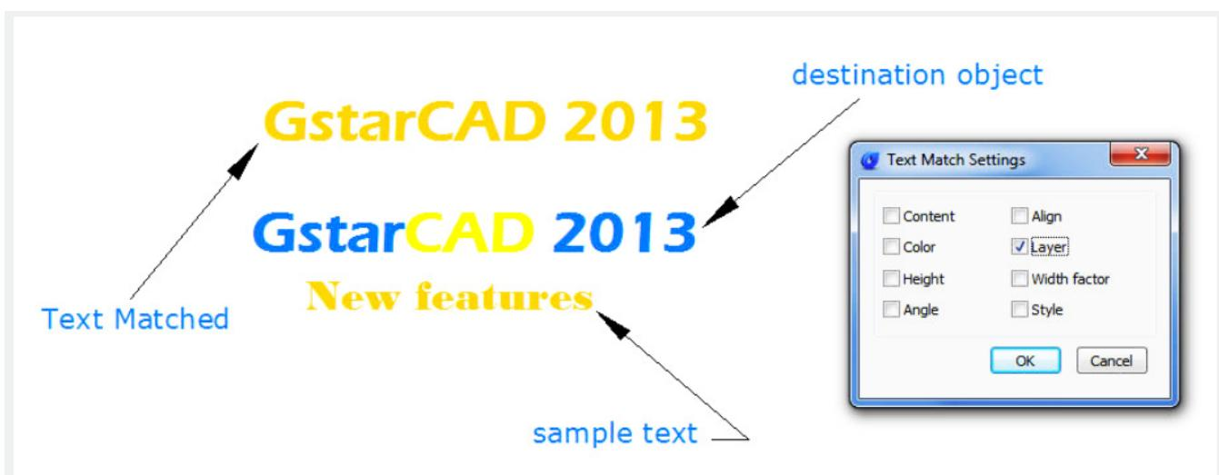
Width factor: Match only the text width factor text frame from the sample text to the destination object(s).
