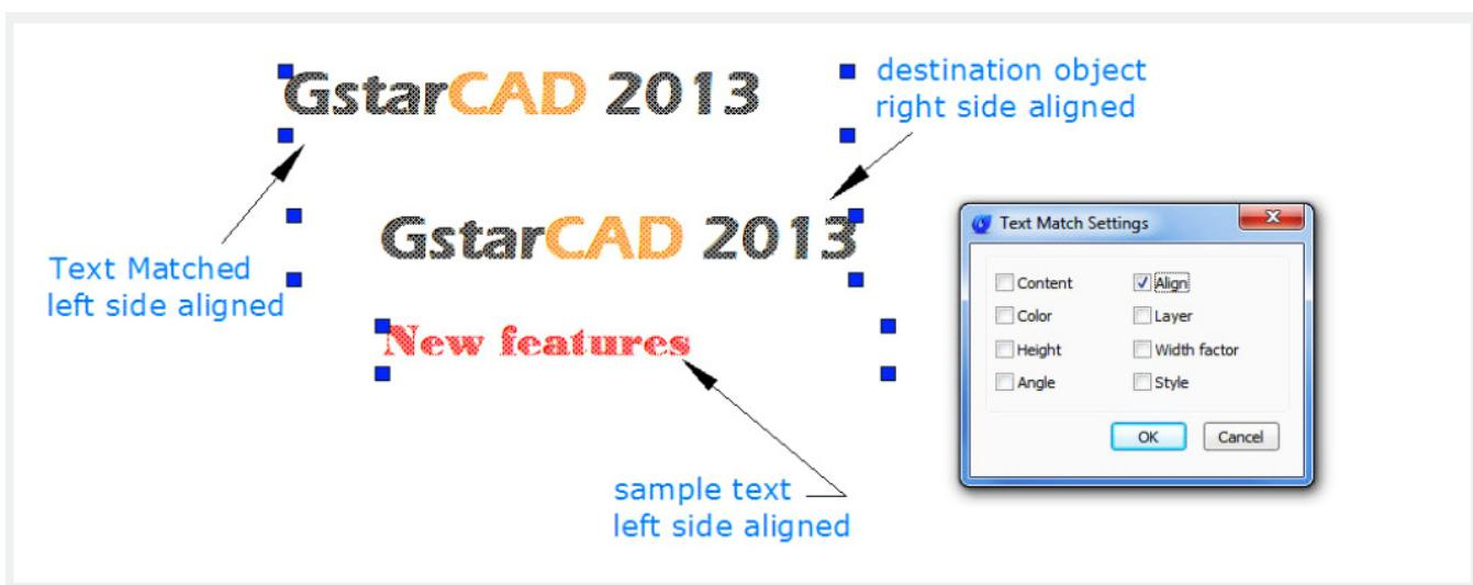
Layer: Match only the text or Mtext layer to which the sample text belongs to the destination object(s).
