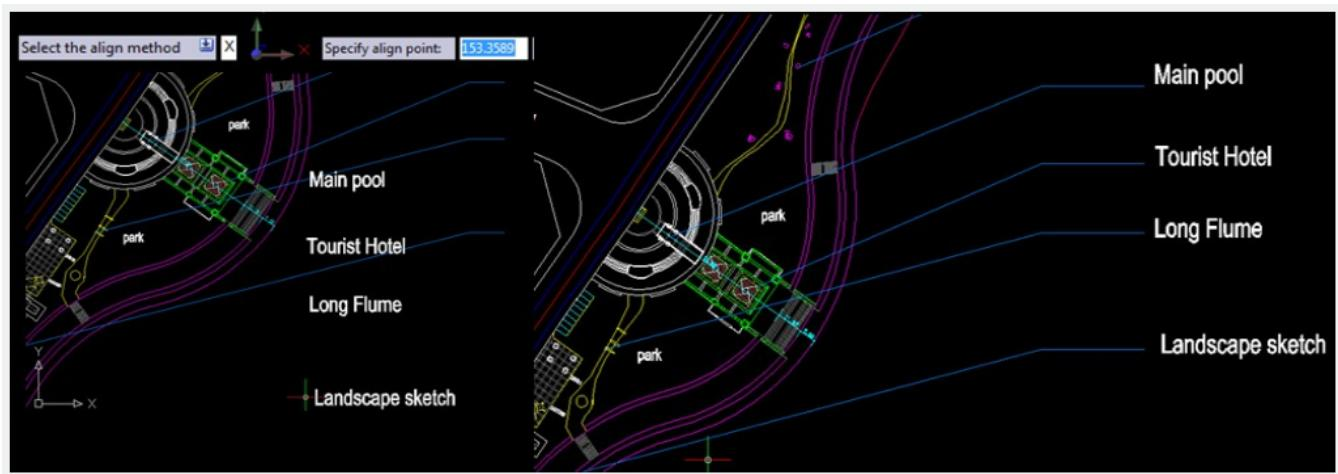
And finally, if we choose the Two points (P) alignment method and then specify two points to align the texts in the correct location (start and end point of Leader). The result is as follows:
