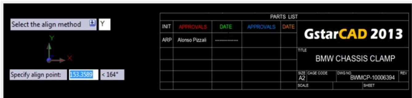
In another example, we choose the X axis alignment method and then specify a point to align the texts in the correct location (end point of Leader). The result is as follows:
