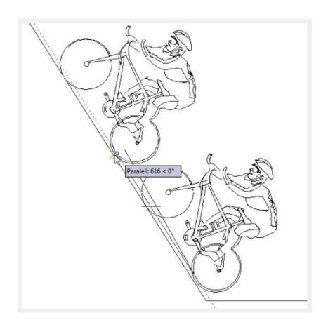
Divide: Linear divide option. Prompts for an additional point and the number of copies to make. Makes evenly spaced copies of the selected objects between the base point and the second selected point.
