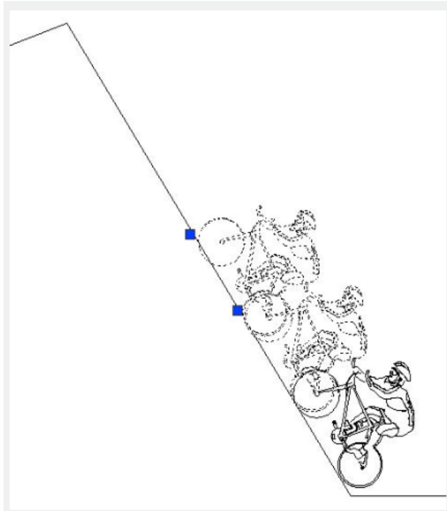
Measure: Linear measure option. Prompts for an additional point and the distance between copies. Makes evenly spaced copies at the specified distance between the base point and the second selected point.
