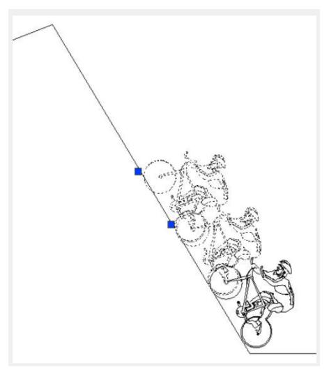
Measure: Linear measure option. Prompts for an additional point and the distance between copies. Makes evenly spaced copies at the specified distance between the base point and the second selected point.
