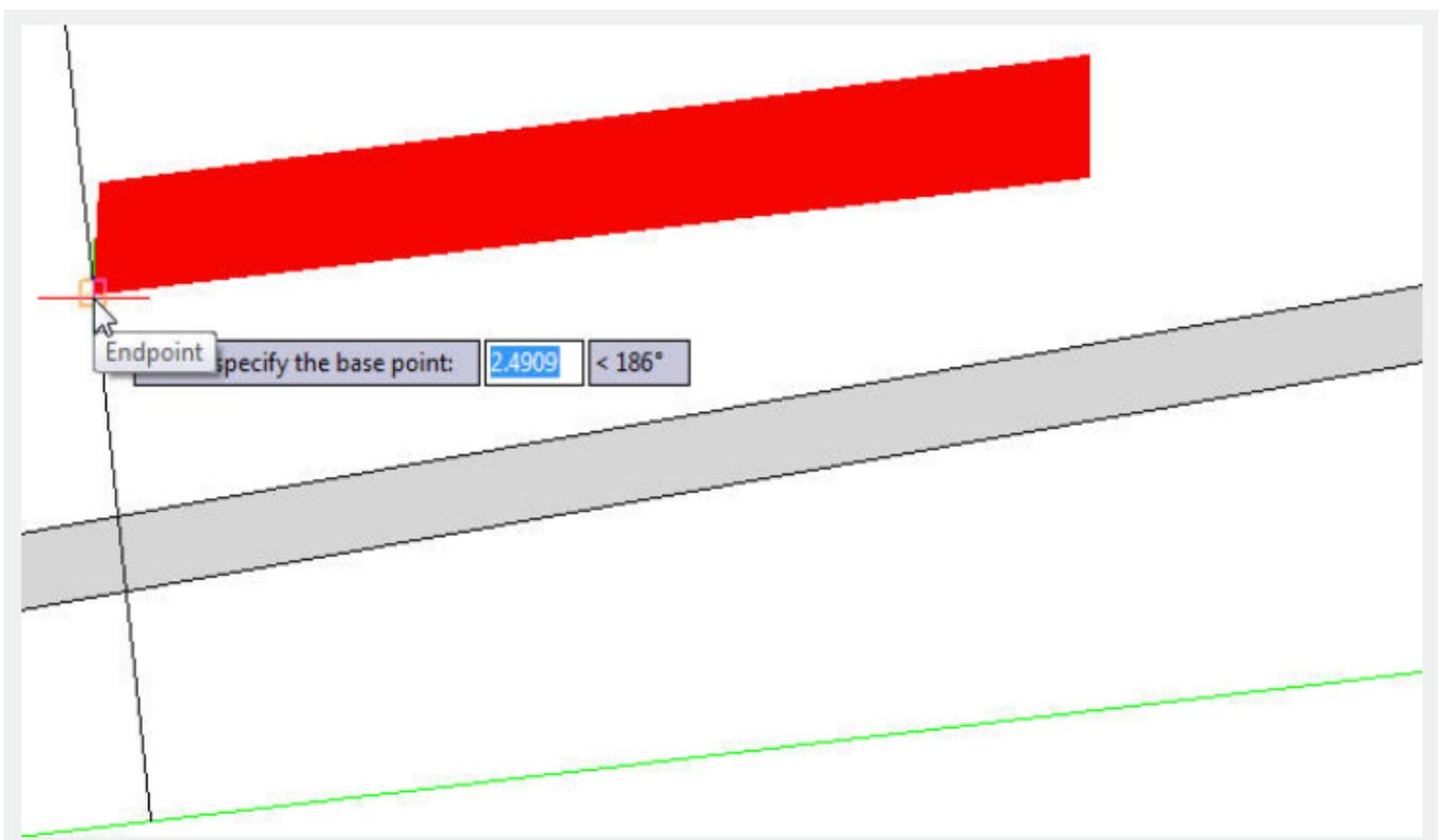
After selecting the base point of the object, a prompt message will be displayed: Specify the object's direction along the curve<Y axis of WCS>:
