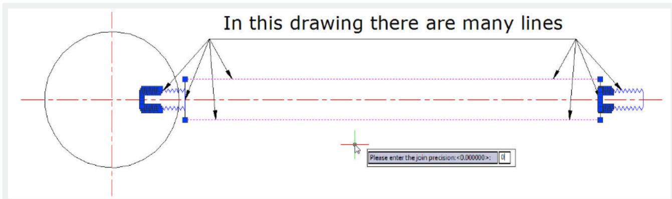
After inputting the join value, Please select the objects to be joined and converted to Polyline:
