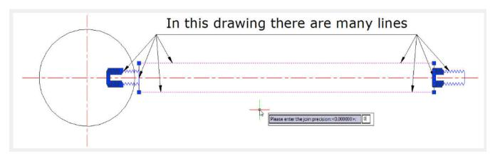
After inputting the join value, Please select the objects to be joined and converted to Polyline:
